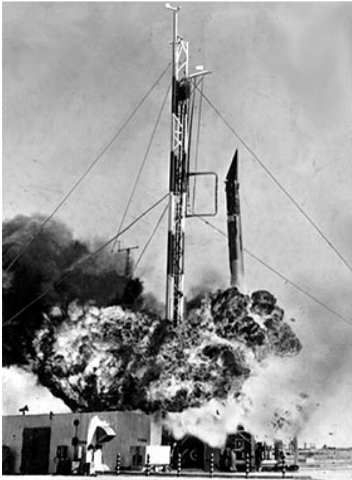
December 6, 1957: Two seconds after launch Vanguard was four feet off the pad. Thrust ceased, it crumpled and then exploded.
